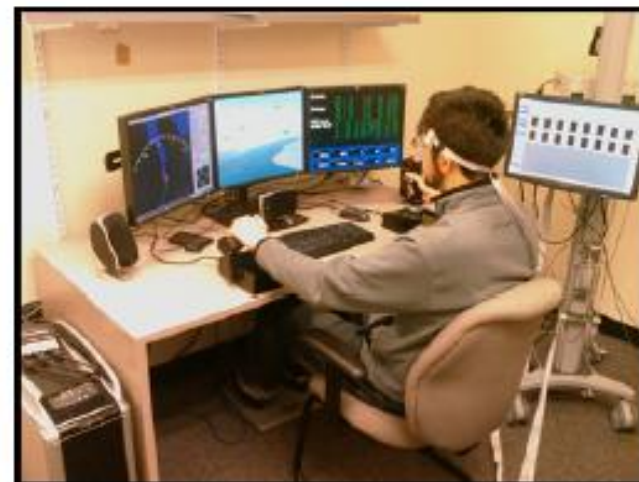
Fig. 3 Subject operating the Predator UAV simulator with fNIR sensor attached and data acquisition apparatus on far right
